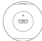
This screwdriver is equipped with a Micro USB universal charging port, and a USB charging cable is included.
